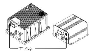
Handset Cable Part Number - 328A1550ATP1 (12 pin plug) Handset Part Number - IC3645LXHS1EC2 (12 pin plug) (includes handset, cable and case) January 1999
