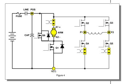
By energizing the transistors in pairs, current can be made to flow in either direction in the field. The field and armature control circuits typically operate at 12KHZ to 15KHZ, a frequency range normally above human hearing. This high frequency coupled with the elimination of directional contactors, provides very quiet vehicle operation.
